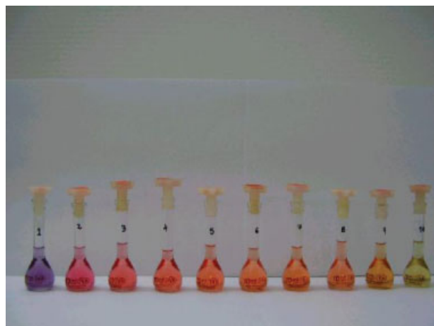
Figure 6. Picture of solutions of the chromium complex 3 in different solvents ordered from left to right according to their increasing \pi^* values: hexane, ether, 2-propanol, ethyl acetate, THF, methanol, acetone, ACN, DMF, DMSO
